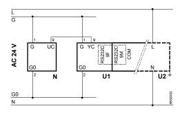
N VAV compact controller U1 Interface converter AST11
