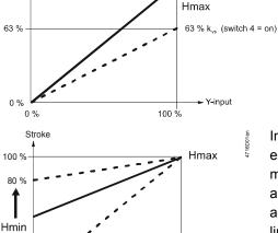
For  $k_{vs}$  reduction (DIL switch 4 in position ON), the stroke is limited to 63% mechanical stroke. 63% of full stroke then corresponds to an input/output signal of 10 V. If, in addition, the stroke is limited to 80%, for example, the minimum stroke is 0.63 x 0.8 = 0.50 of full stroke.
