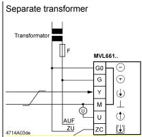
Terminal assignment for controller with 3-wire connection
