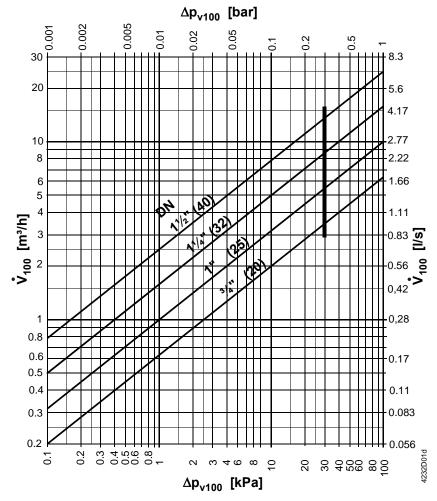
$\Delta p_{\text{max}}$  = Maximum permissible differential pressure across the slipper valve's control path, valid for the entire actuating range of the motorised slipper valve
